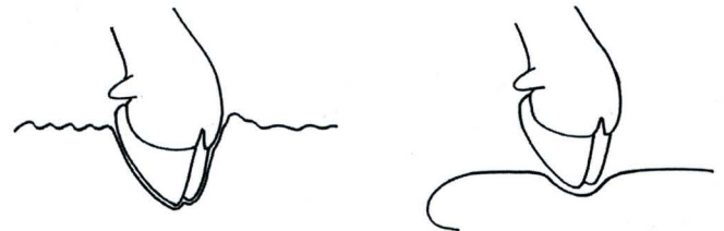
Figure 3. Compare how the toe of the main weight-bearing limb of the cow interacts with the stall surface during rising and lying movements. The cushion and traction of sand is in stark contrast to the small surface area of contact on a mat or mattress stall.
