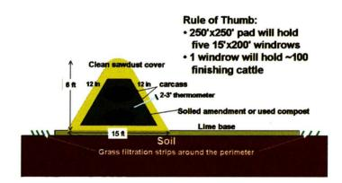
Figure 4. Schematic of composting windrow (intact carcass)
