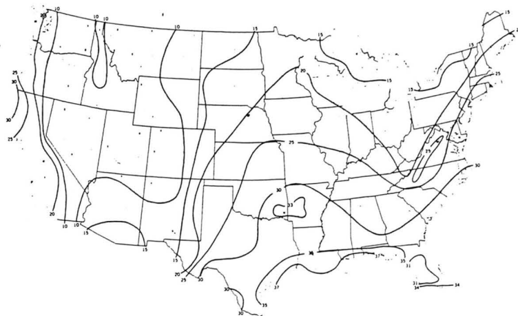
Exhibit 2. Annual runoff from unsurfaced feedlots (CN-90) as percent of precipitation for the year.
