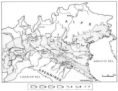
Fig. 5 - Schematic lithologic map of the Po Valley and surrounding areas. Legend: 1) gravels and coarse sands with high productivity aquifers; 2) sands and subordinate gravels and silts with high to low productivity aquifers; 3) silts, clays and subordinate sands with low to very low productivity aquifers; 4) Alpine and Apennine bedrocks; 5) main water courses; 6) lakes; 7) main wells for water-supply purposes.
