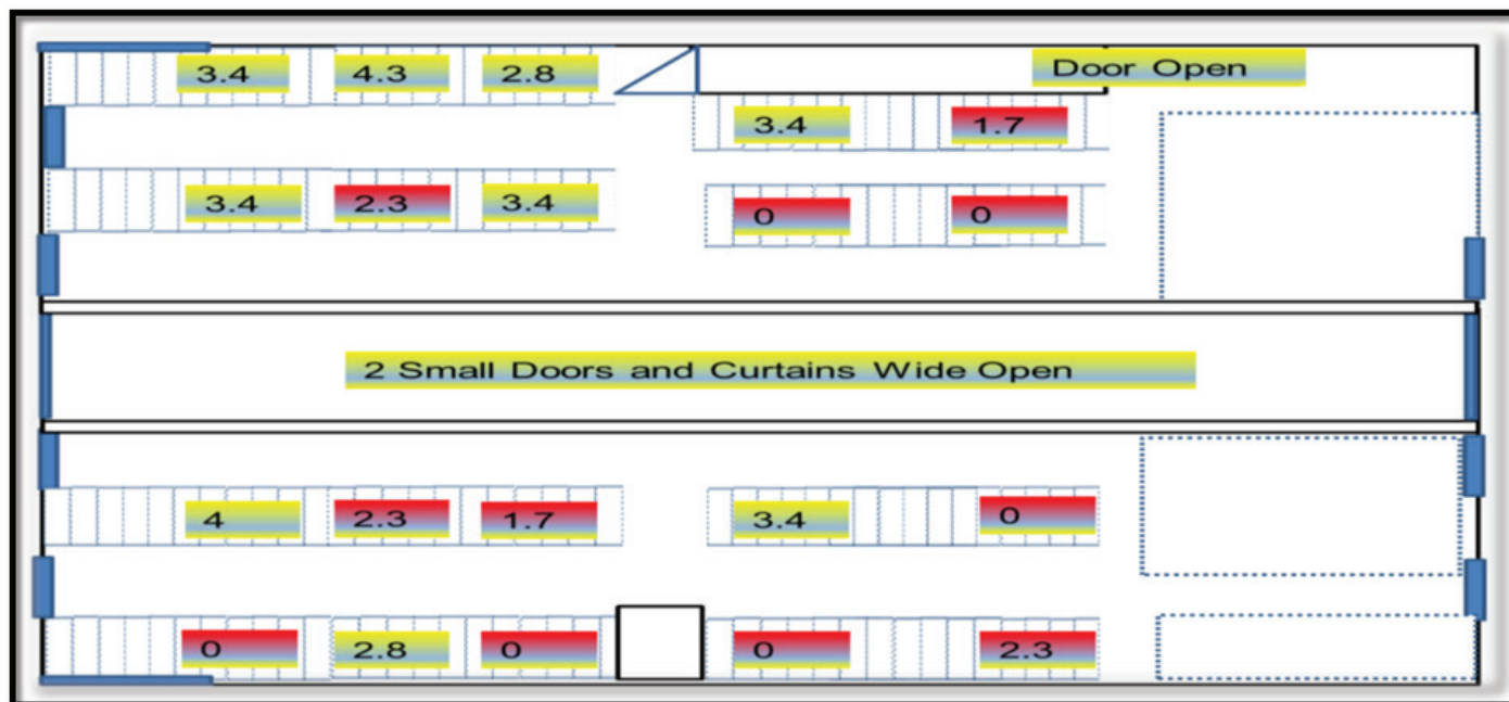
Figure 3. An example of a wind tunnel analysis map. Numbers are denoted in MPH. Minimum target is >2.5MPH. Picture created in PowerPoint.
