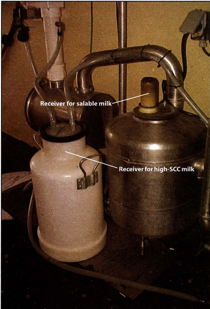
Figure 5b. Vacuum source for high-SCC milk receiver.
