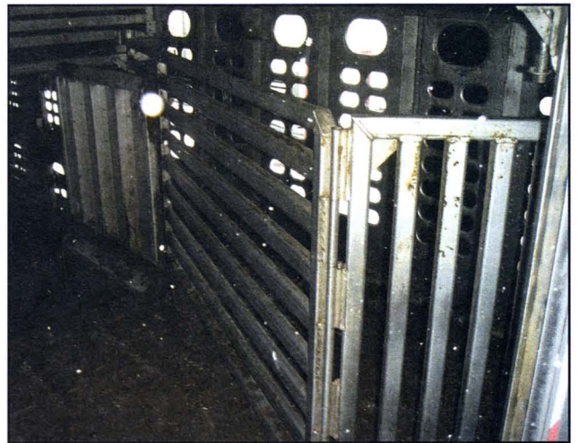
Photo 5. Truck gates used to guide cattle to exit.
