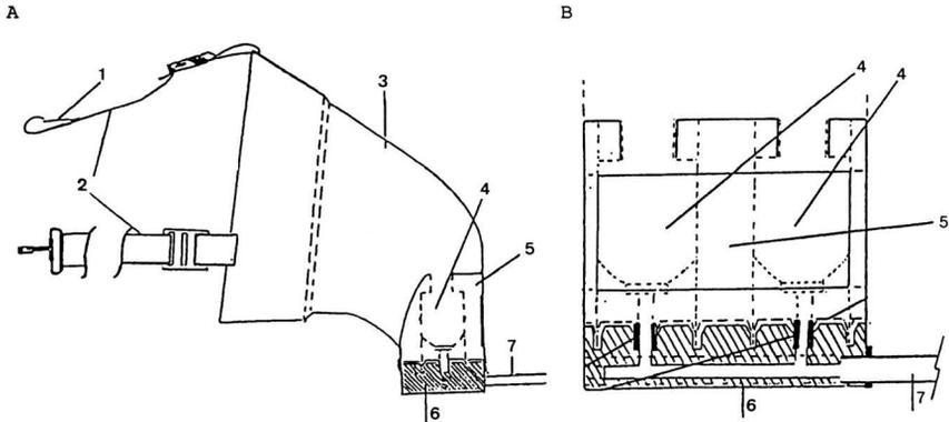
1 = Clip; 2 = Strap to attach the mask; 3 = Face mask; 4 = Jet nebulizer; 5 = Aerosol generating chamber; 6 = Nebulizer supporting plate; 7 = Feeder pipe of compressed air.
