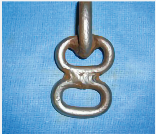
Figure 2: A welded 3-link clevis that allows for use of the nylon webbing as a lift wrap at the level of the gastrocnemius tendon.
