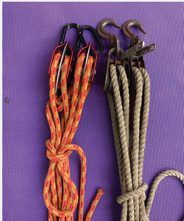
Figure 5: A block and tackle or fence stretcher apparatus if doing a lot of foot work.
