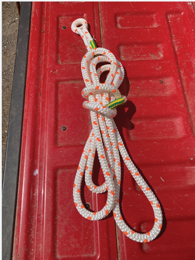
Figure 3: Fifteen-foot (5 meter) lengths of 12- to 18-strand woven arborist rope, either ½ inch or 5/8-inch diameter.
