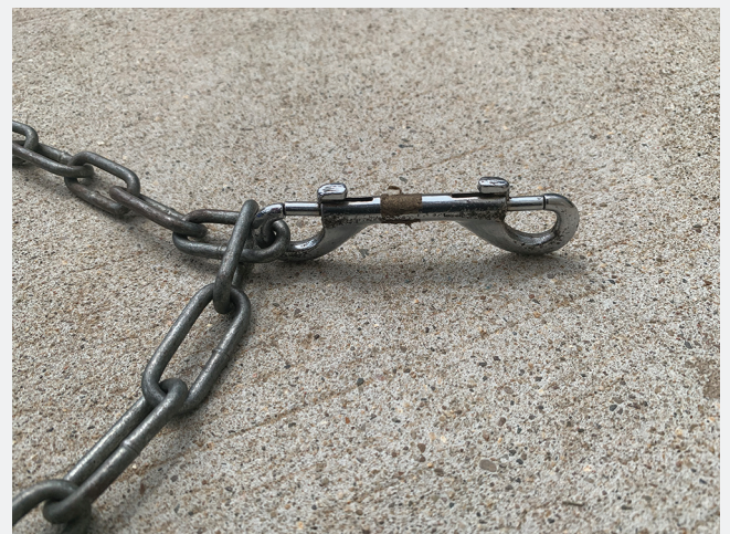
Figure 2: Lengths of chain with links of a size that allows one link to slip inside the diameter of another link.
