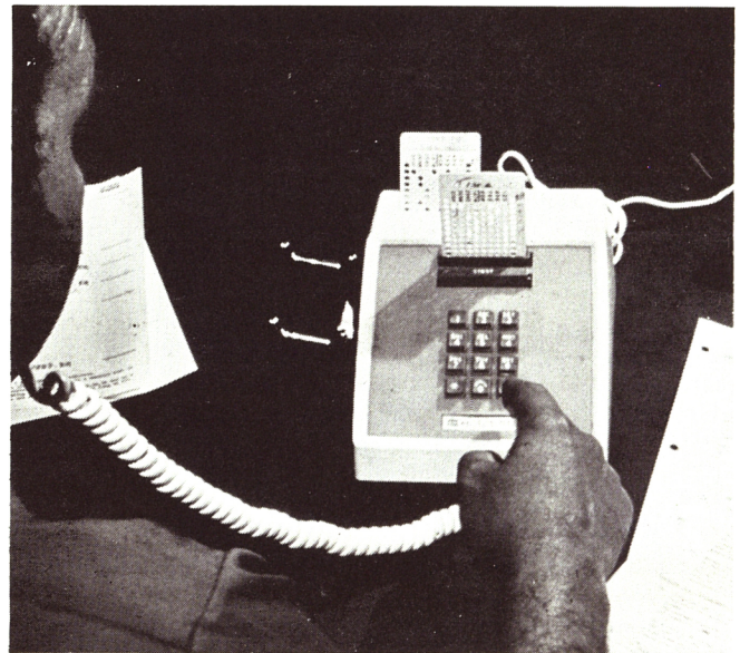
Figure 2. A telephone is used to contact the computer in Ann Arbor, Michigan, with information on analysis and cost of available feeds along with animal consumption and production data. The computer formulates a least-cost balanced ration based on the data supplied and provides the dairyman with specific recommendations for feeding his herd including the cost of the ration. (Photograph courtesy of Dr. Don Hillman.)
