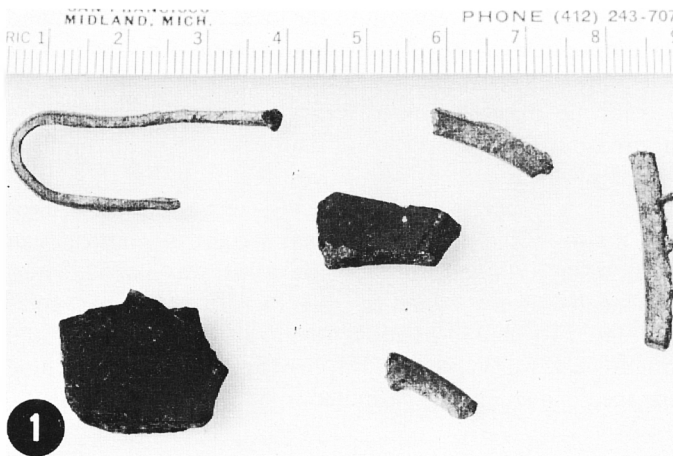
Figure 1. Black plastic like material and U-shaped solder bar believed to be parts of the chopped up discarded tractor battery. Chemical analysis determined these fragments to be pure lead.
