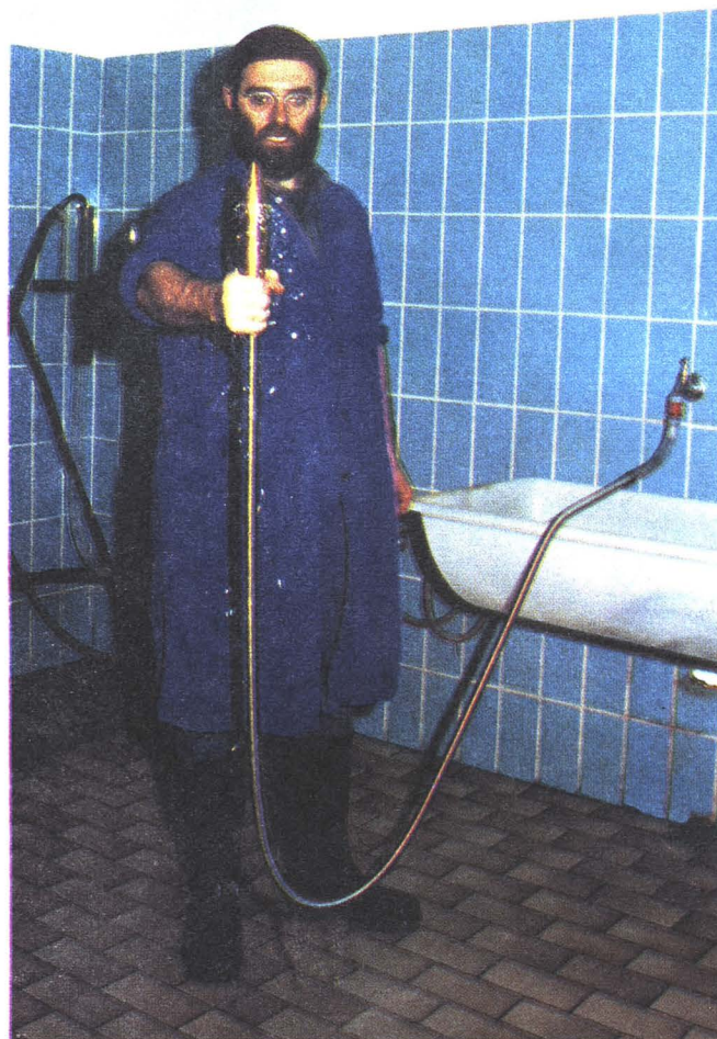
Figure 5. Cleaning of the probe by connecting it to a water tap
