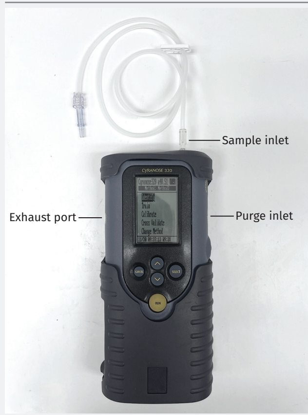
Figure 1: Cyranose 320®* eNose with labeled features used for sample collection.
