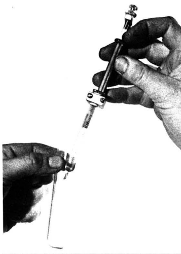
Fig. 1.1. 1 ml. urine plus 5 drops chloride indicator plus 3 dropperfuls .1N HNO 3
